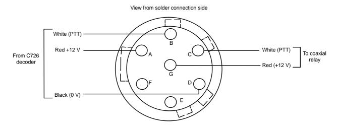
Figure 2: Wiring details for the 7-way male connector
